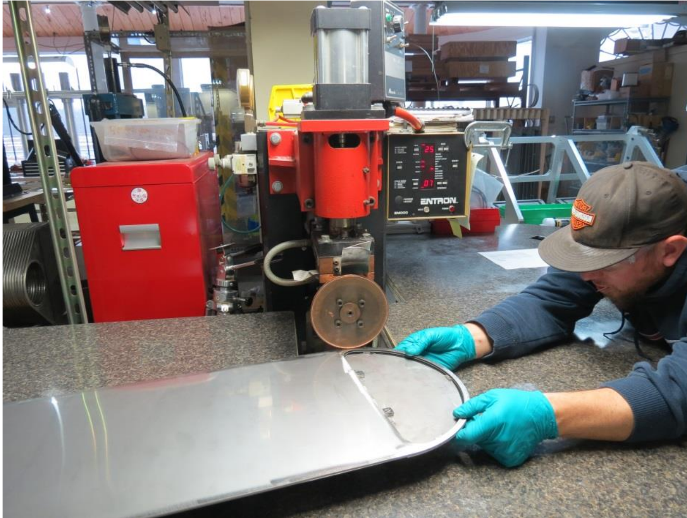
Resistance weld parting sheets to edge bar pressure boundary
