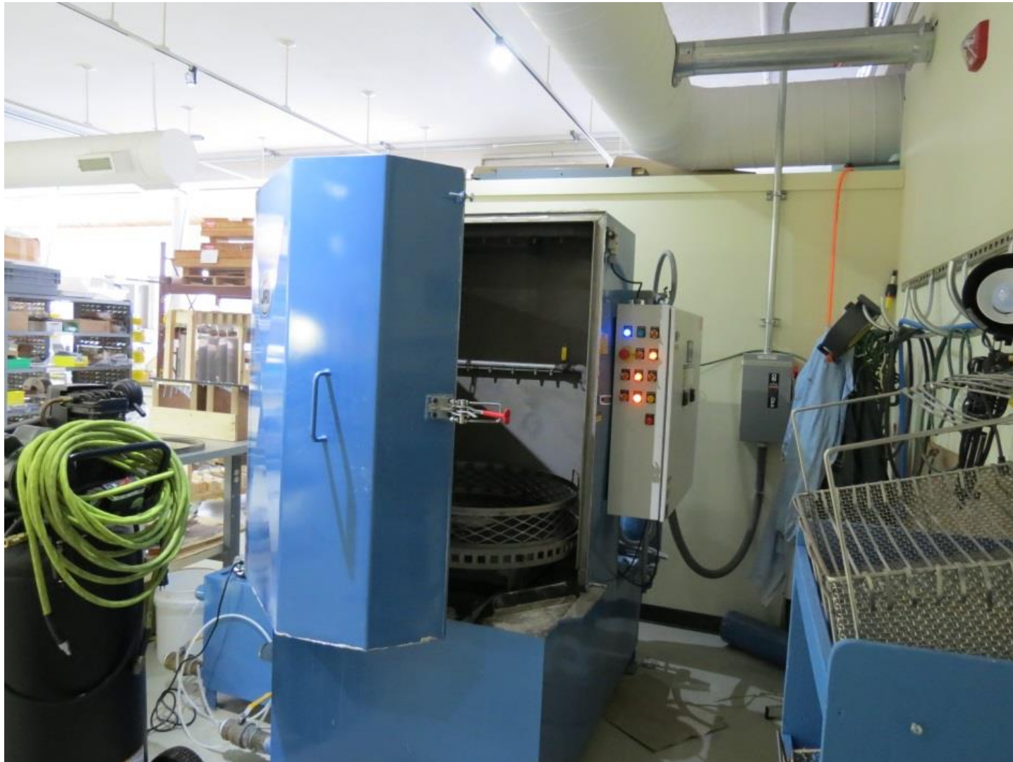
Cabinet Spray Washer. High pressure jets aqueous degreaser solution.
