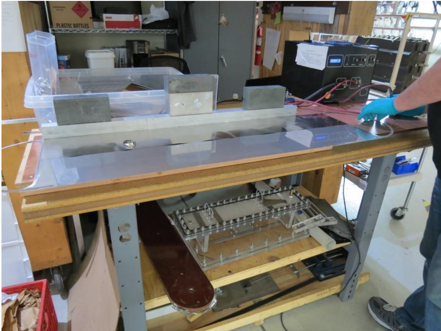
Light energy tack weld to apply foil onto parting sheets
